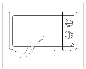
f i When measuring near a corner of the door, keep the probe perpendicular to the areas making sure the probe end at the base of the cone does not get closer than 2 inches from any metal. If it does, erroneous reading may result.
